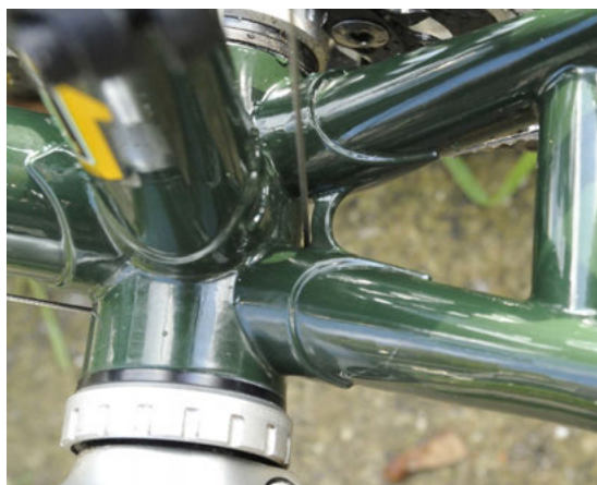
ABOVE: Reynolds 631 fork blades. The crown has reinforcing ribs around the steerer tube. Also, note slimline Kool Stop pads on the generous braking surface.
